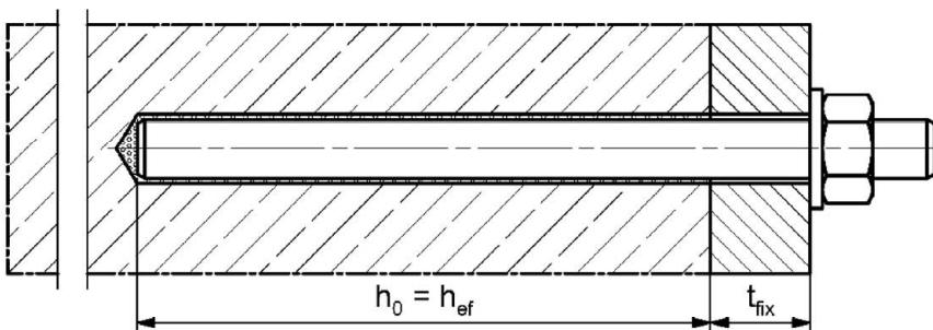
Push through installation (annular gap filled with mortar)
